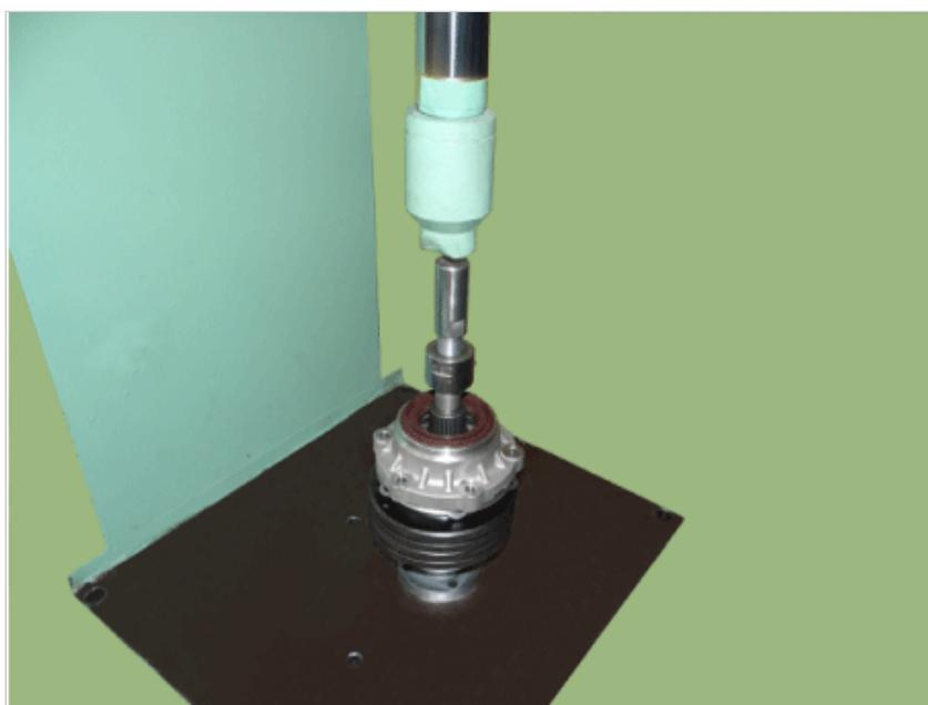
4. Remove the pinion oil seal (A) & pinion front bearing from the pinion cage by a screwdriver.
