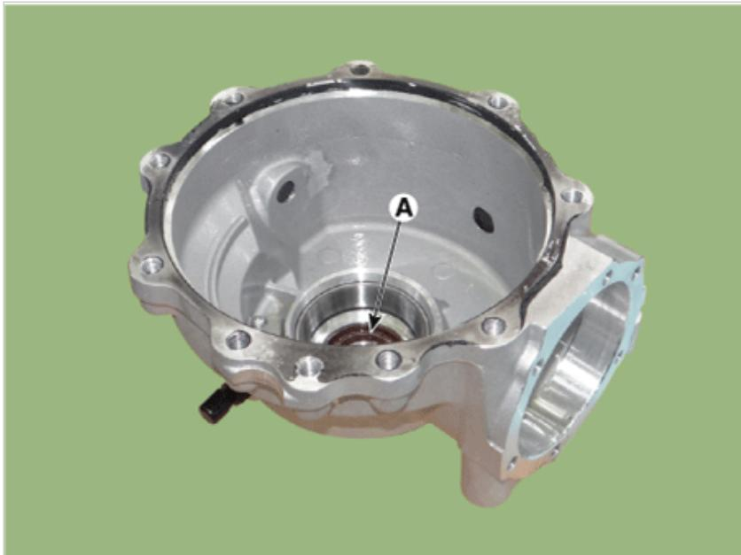
8. Using the SST (09452-2W300), remove the spacer & bearing race from the differential carrier.
