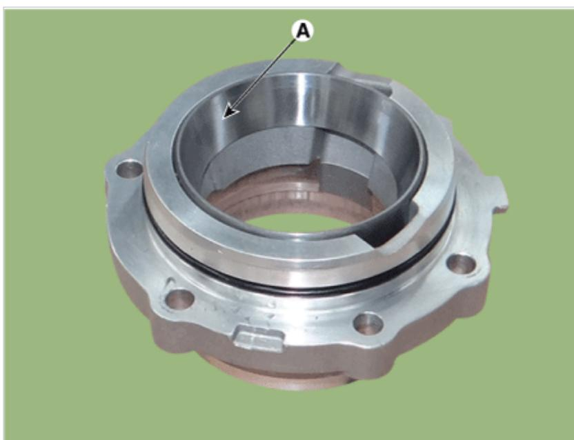
6. Separate the pinion bearing spacer(A) and pinion front bearing(B).
