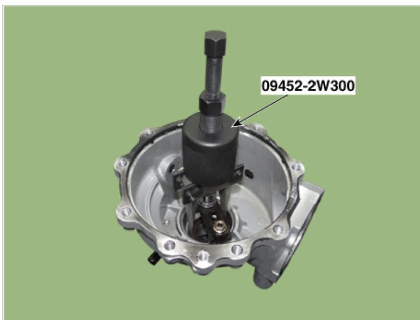
9. Using the SST (09474-4E200), remove the side bearing.
