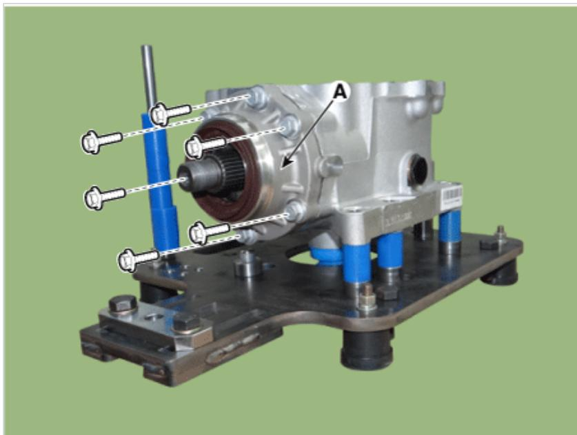
3. Remove the pinion drive gear from pinion Drive gear assembly using a press.
