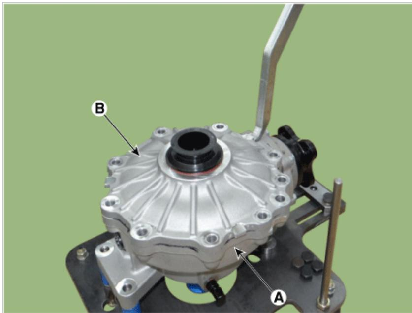
5. Remove the spacer (A), side bearing race (B) using a hammer and chisel.
