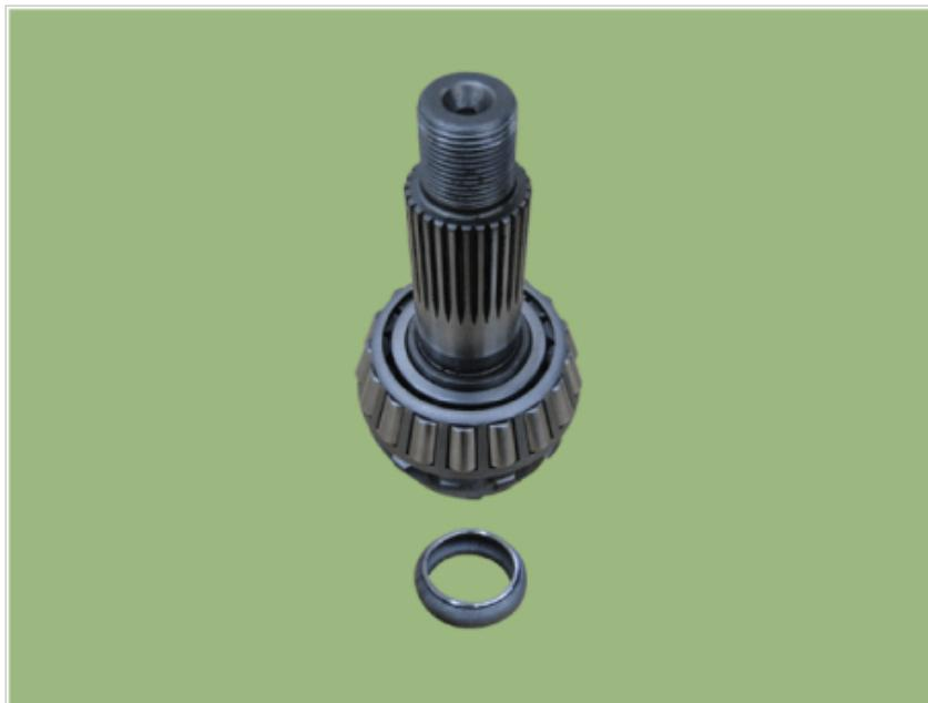
7. Using a press, remove the pinion rear bearing.
