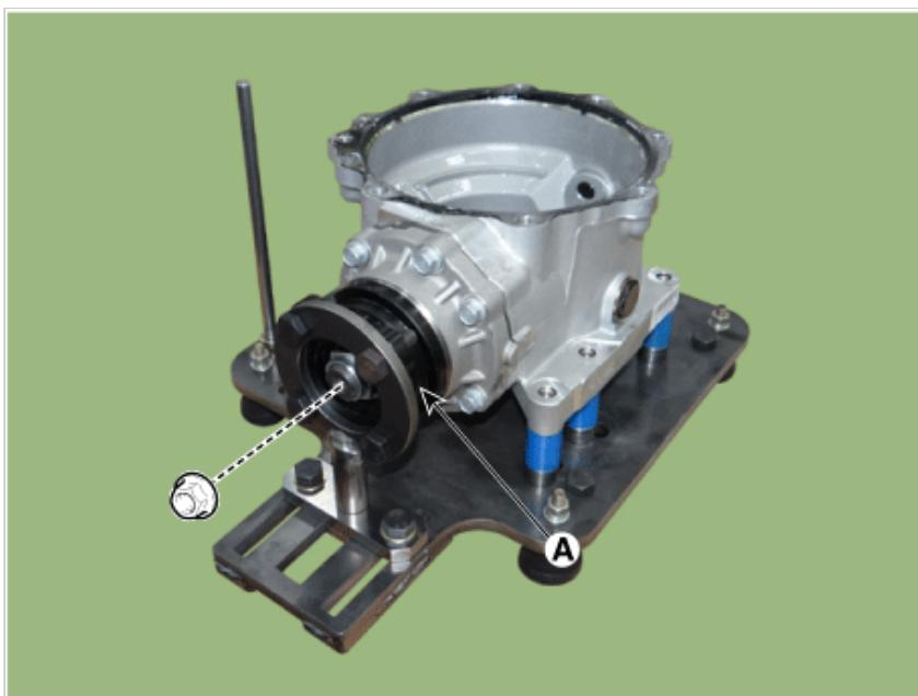
2. Loosen the bolts and remove the pinion cage(A).
