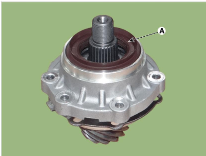
5. Using a hammer and chisel, remove the pinion rear bearing race (A).
